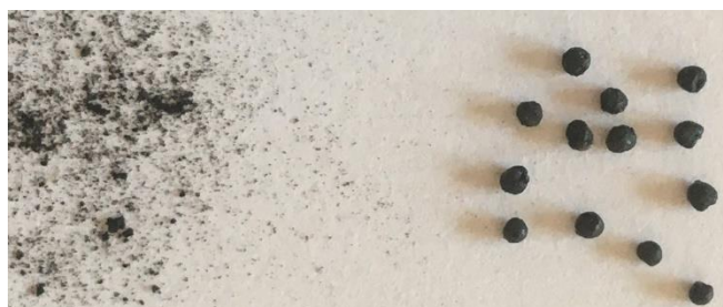
Fig. 7. The image of \text{CoFe}_2\text{O}_4 particles (left) and \text{CoFe}_2\text{O}_4 -Chit particles (right)
