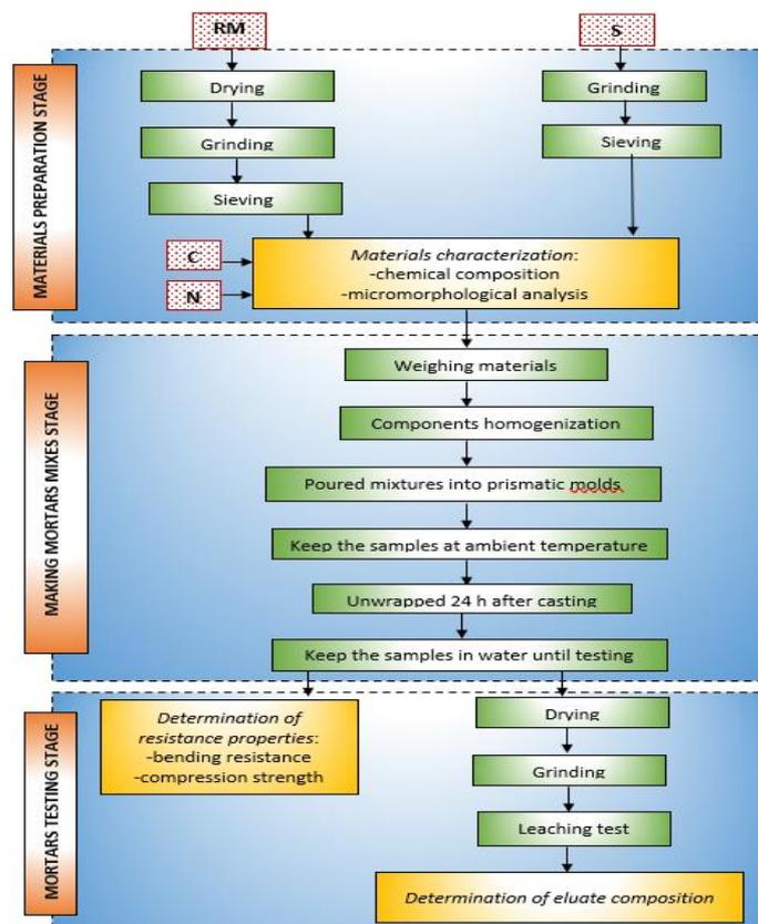
Fig. 2. Flow diagram of the experimental program stages
